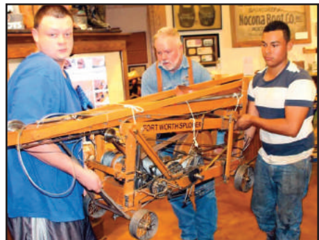
Operational replica of a spudder
